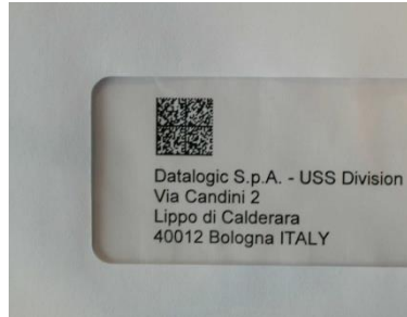
Figure 18 - Address Coded in Data Matrix Symbology for Automated Mail Processing
