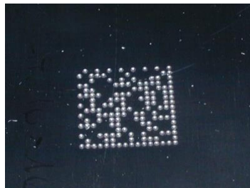
Figure 24 - Directly Marked Dot Matrix Code Characterized by Outstanding Separation Distance between Adjacent Code Elements
