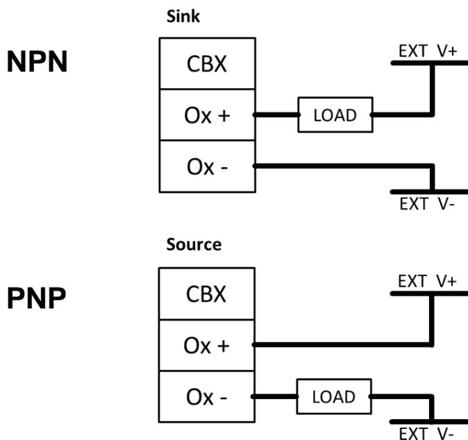
Figure 31: Unpowered Outputs
