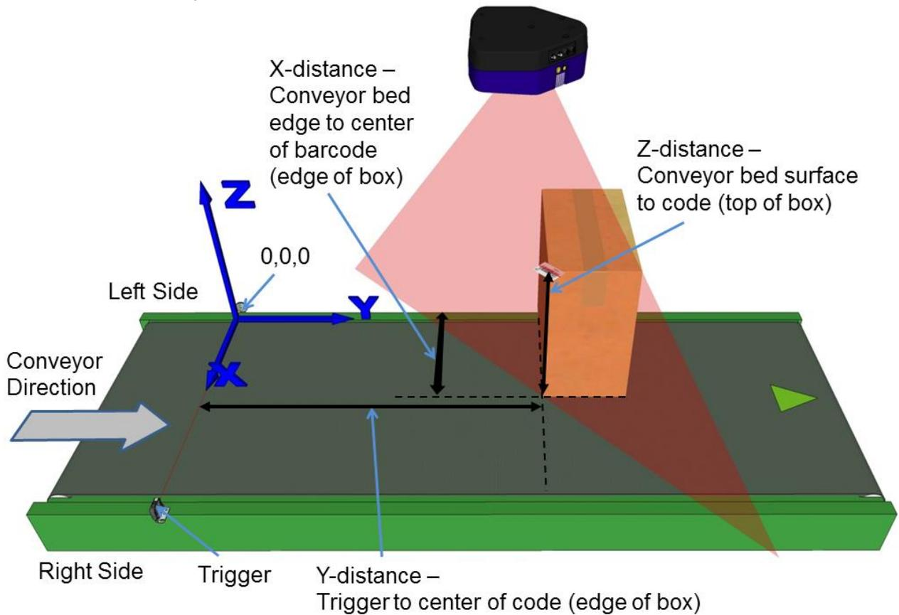
Figure 47: Top-read leg 2- 1<sup>st</sup> barcode placement
