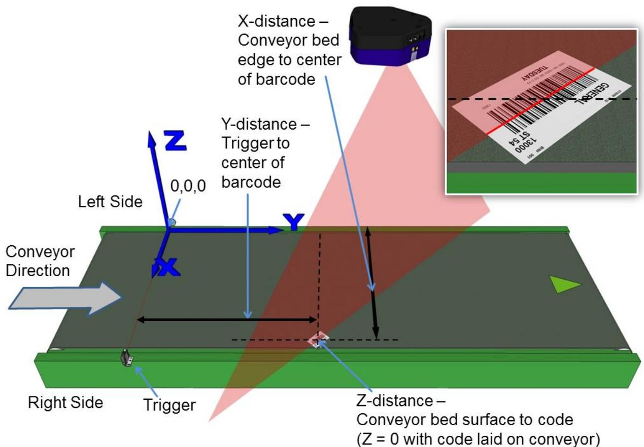
Figure 45: Top-read 2<sup>nd</sup> barcode placement
