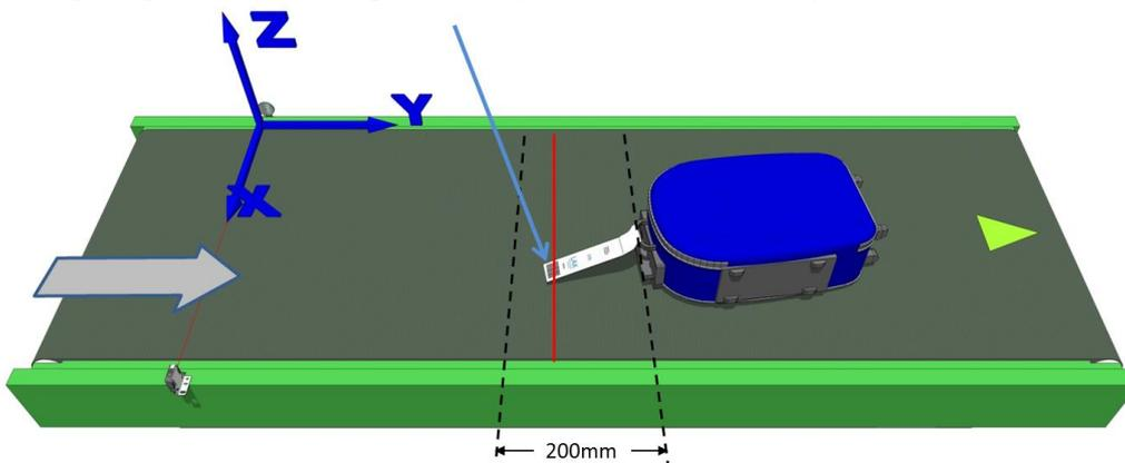
Figure 68 – Compensating for Irregular-Shaped Packages
