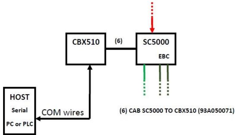
Figure 66 – Large Synchronized Network with COM to Host
