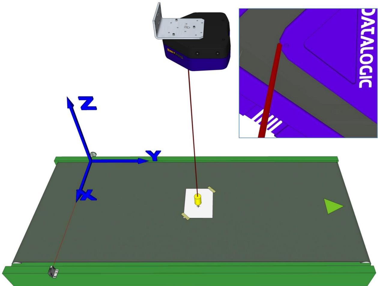
Figure 58: Using a plumb bob to mark scanner location on conveyor
