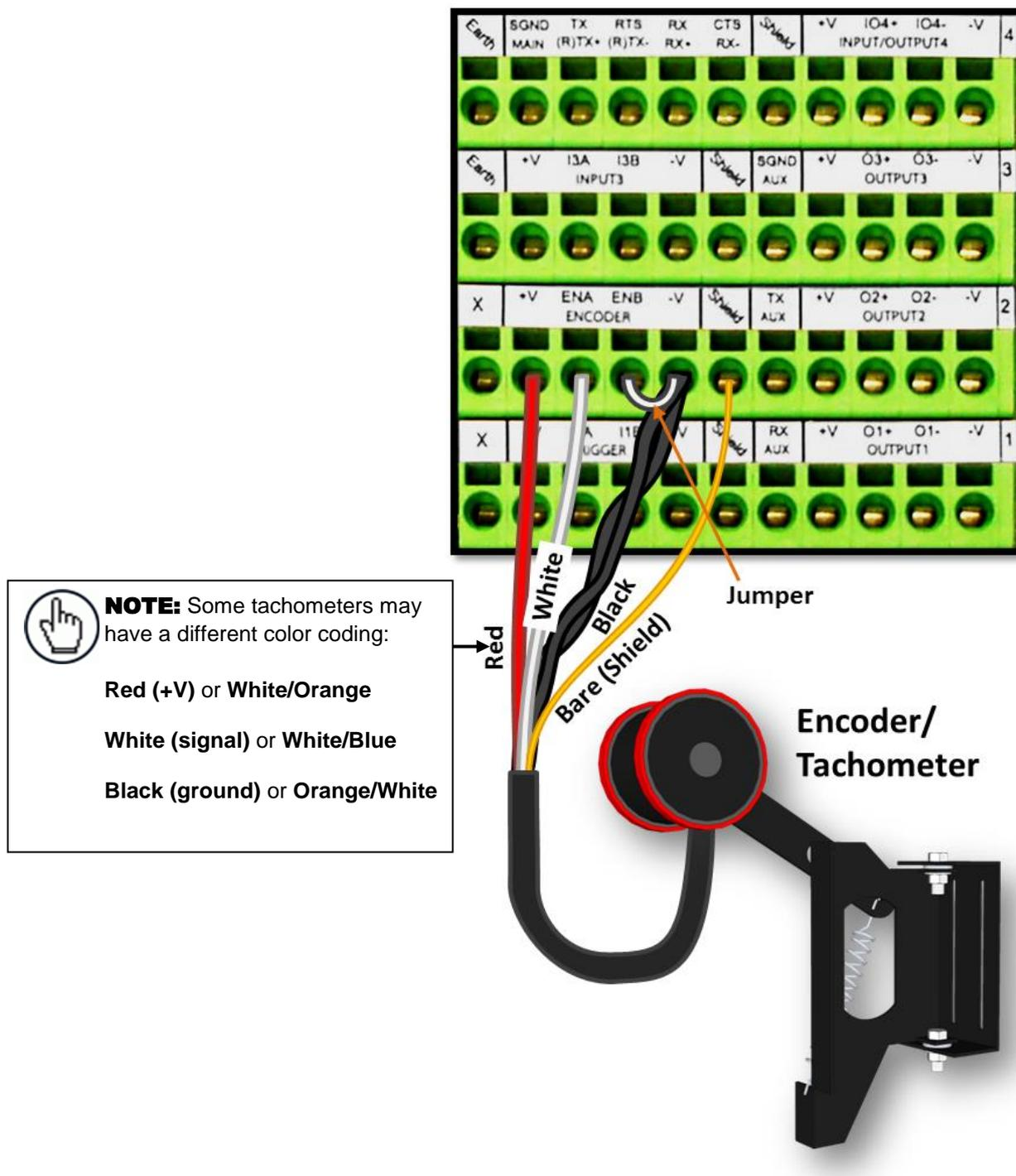
Figure 28: OEK-2 (93ACC1770) Encoder/Tachometer Wiring (PNP Output)
