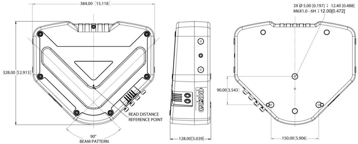
Figure 12: DX8210 Overall Dimensions
