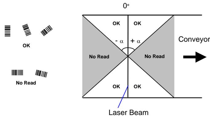
Figure 72 – Reading Zones with  $\alpha$  Max
