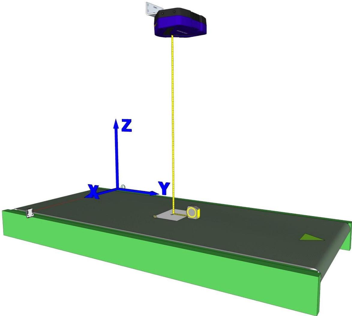
Figure 61: Measuring the Z Offset
