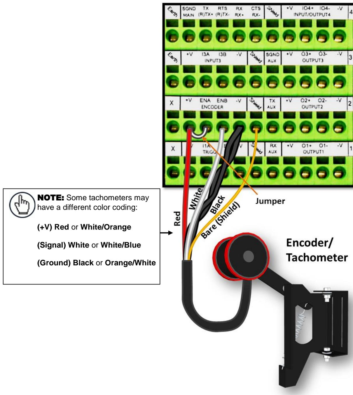
Figure 26: OEK-2 Encoder/Tachometer Wiring (NPN Output)
