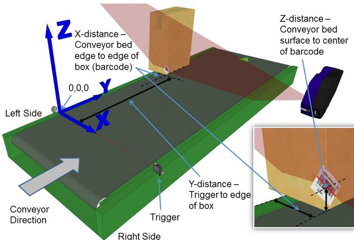
Figure 50: Side-read 1<sup>st</sup> barcode placement
