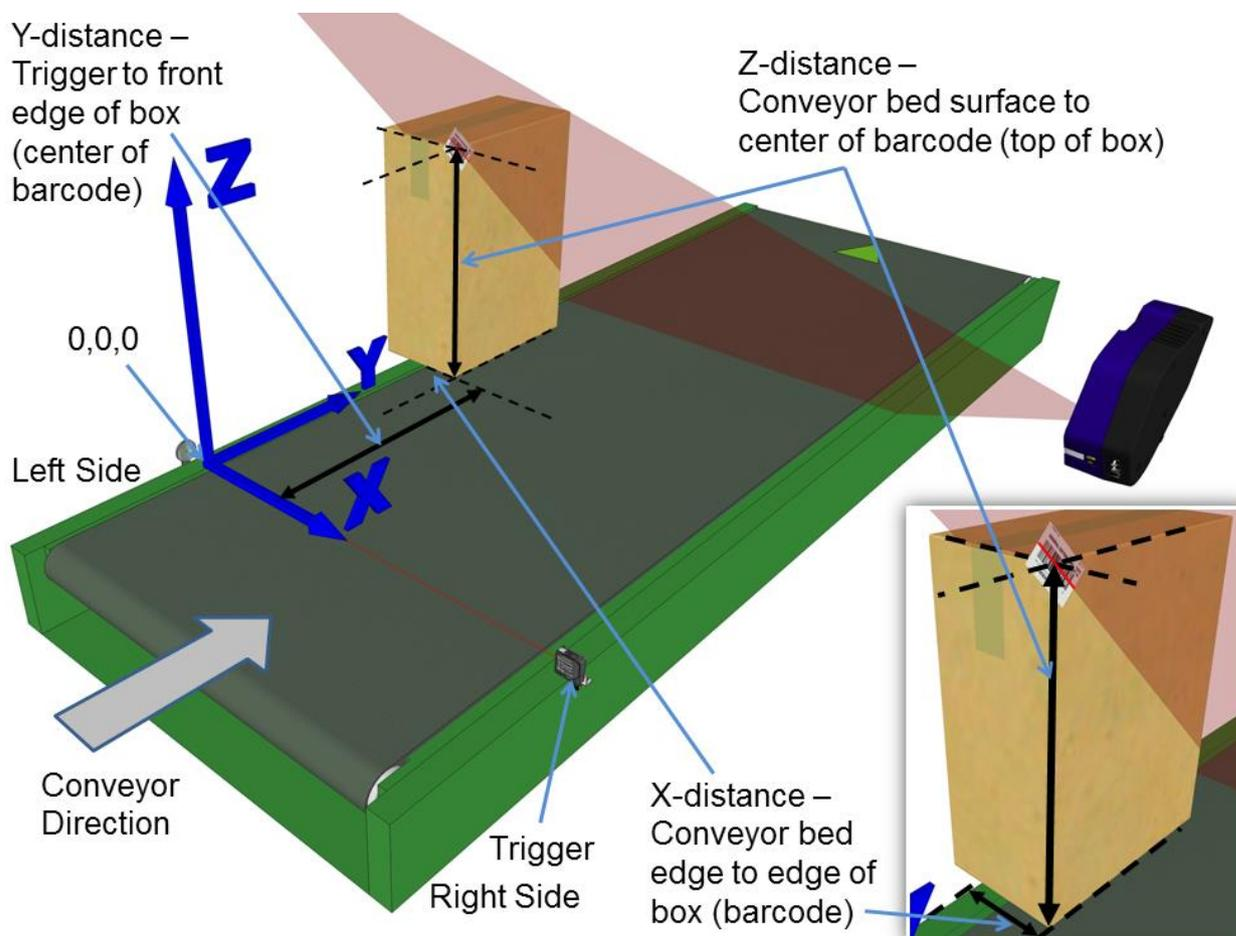
Figure 52: Side-read 2<sup>nd</sup> barcode placement
