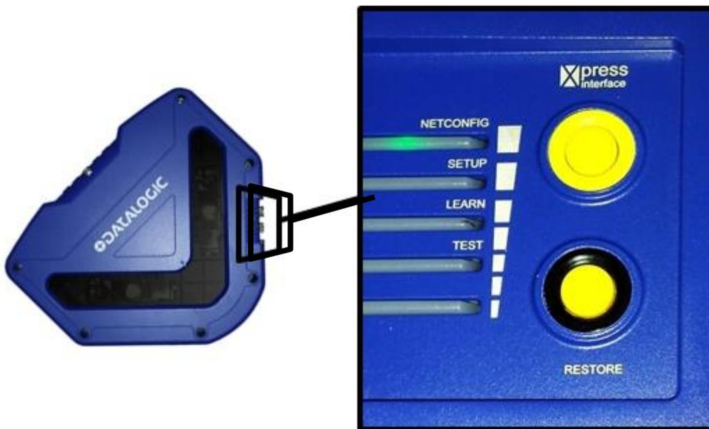
Figure 37: Control Panel Buttons
